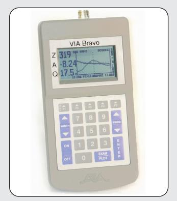
AEA's **VIA Bravo** is a TRUE, Hand Held, Vector Impedance Analyzer that is Impedance independant. This means you can measure any circuit or antenna Z from 10 to 2000 Ohms. The analyzer has the capability of providing accurate measurements of **Z**, **X**, **R**, **Phase Angle** (0.5 degree resolution), **Q** (3dB curve points), **SWR** and **Return Loss**, as well as **TDR** and **Spectrum Analyzer** modes! The Q calculation works for both parallel and series resonances.
